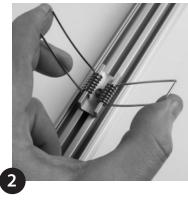
Slide/fix spring clips into required position with screw, then hold under tension folded-up ready to fit into slot.
